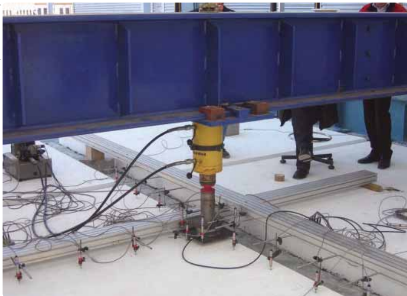
Figure 1: Load testing of a steel-fibre-reinforced concrete slab at Greenwich University.
