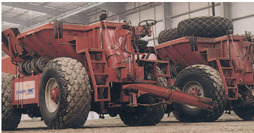
Figure 2: Twintec's low-pressure concrete dumpers.
